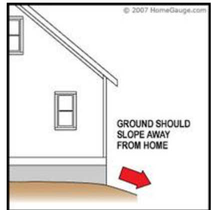
2.4 Picture 3 Ground should slope away from home, 1" per foot for at least 6 feet
